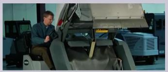
The hopper's safety bar control is located in the cab, maximizing the likelihood of operator use and improving safety.
