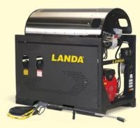
**SLX:** The industry's biggest and only portable hot water pressure washer that delivers 200°F water at a rate of up to 10 GPM, plus supports a 2-gun operation. The 3 models of the extra-rugged, skidmounted SLX are powered by gasoline or diesel and feature the Landa Pump with 7-year warranty.
