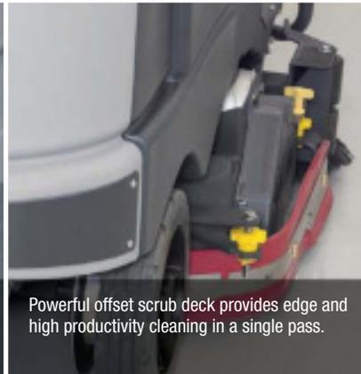
Powerful offset scrub deck provides edge and high productivity cleaning in a single pass.
