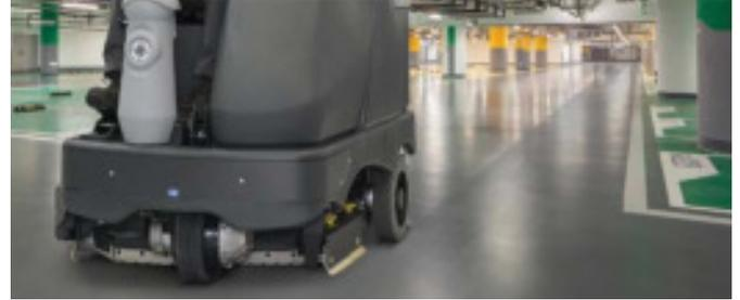
With the tightest aisle turn in its class and large, 70 gallon solution and recovery tanks to maximize scrubbing time, the SC6500 helps you get the job done faster. And, with a high power scrub deck, a single pass is all you need to get an amazingly clean floor.
