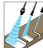
Rotary nozzles clean deep like a 0° nozzle but fast like a 25° nozzle
