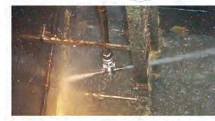
CLEANING RANGE: UP TO 75' PRESSURE: 50-300+ PSI FLOW: 40-120 GPM IMPACT: UP TO 30 LBS AT 25'
