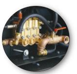
▲ Industrial-duty tri-plunger Landa Pump designed to run at low RPM for long life, 7-year warranty, with single-rail true-track Pulley Adjustment.
